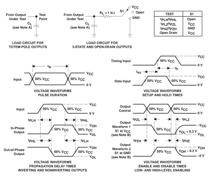
NOTES: A. C<sub>I</sub> includes probe and jig capacitance.
